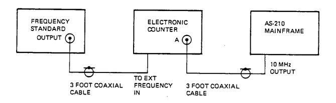
Figure 5.1 AS210 Internal Frequency Standard Test Configuration
