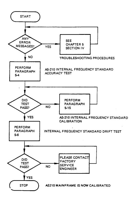
Figure 5.3 Flow Diagram of the Calibration/Alignment Procedure for the AS210 System Mainframe
