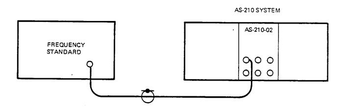
Figure 5.2 AS210 Internal Frequency Standard Drift Test Configuration
